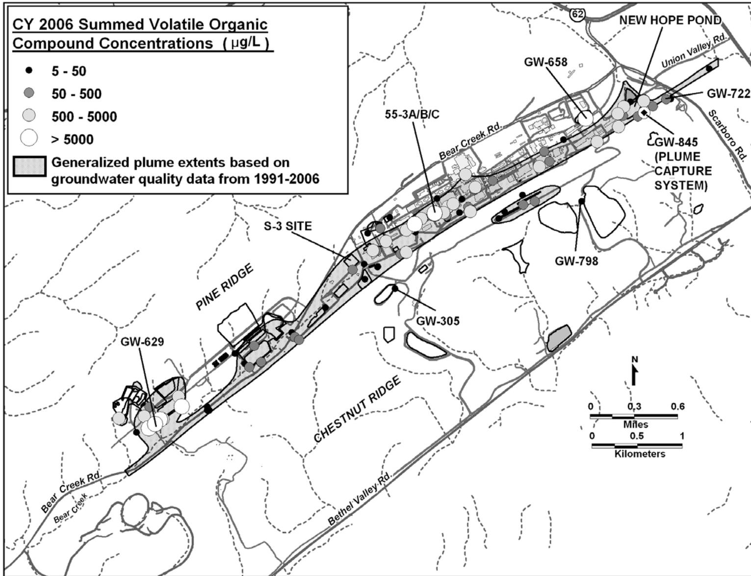
Fig. 6.20. Summed volatile organic compounds observed in groundwater at the Y-12 Complex, 2006.
