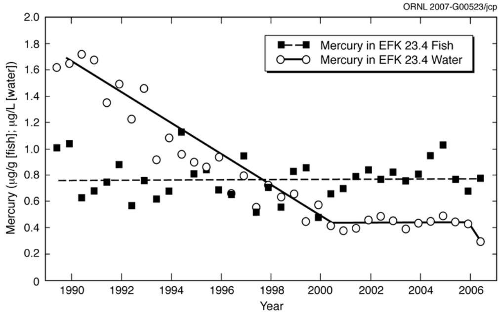
Fig. 6.10. Semiannual average mercury concentration in muscle fillets of fish and water in East Fork Poplar Creek at Station 17 through spring 2006. (EFK = East Fork Poplar Creek kilometer.)
