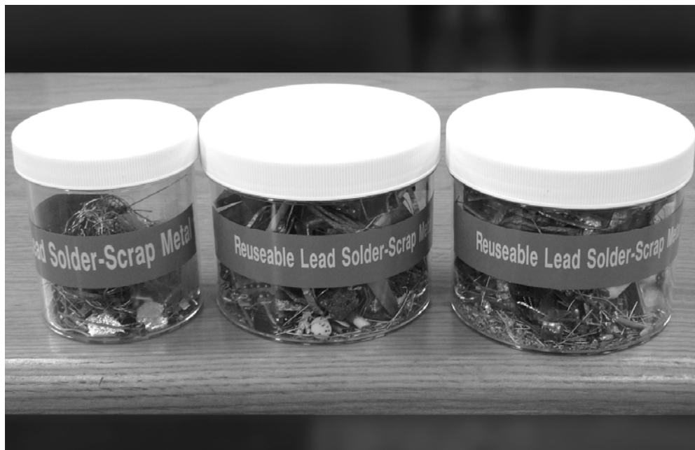
Fig. 5.7. Example of reusable lead solder-scrap metal.
