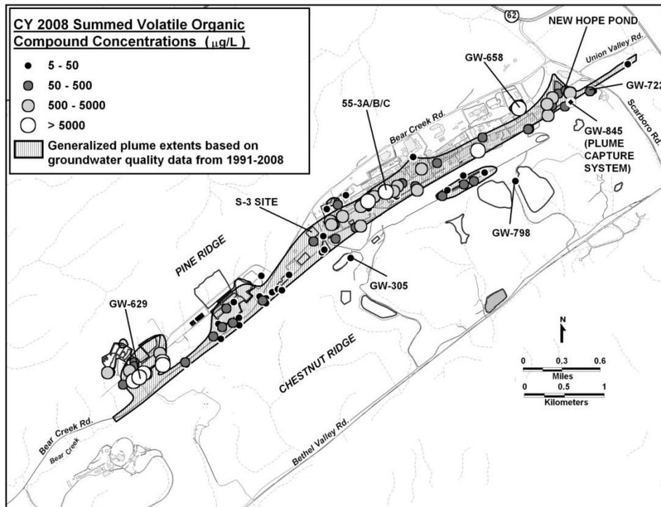
Fig. 4.37. Locations of Y-12 Complex perimeter/exit pathway well, spring, and surface water monitoring stations.
