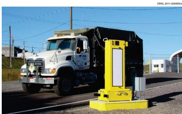
**Fig. 3.7. Truck carrying a waste shipment passing through an electronic tracking station, part of the Radio Frequency Identification Transportation System, en route to the Environmental Management Waste Management Facility.**
