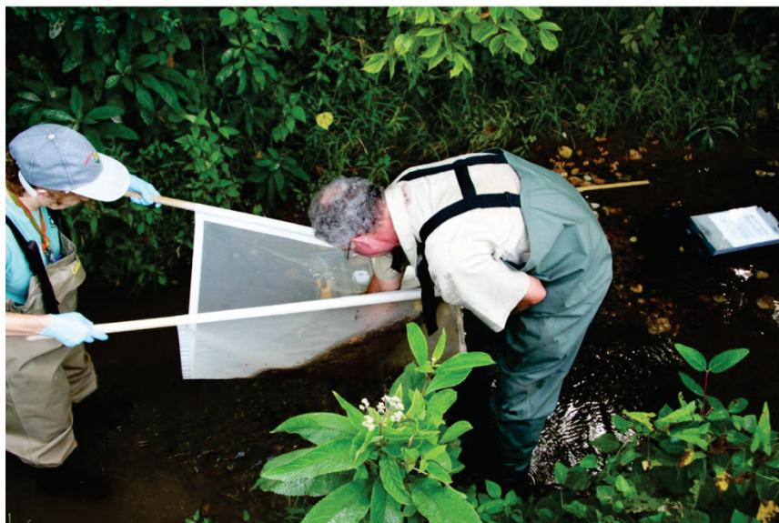
**Fig. 3.57. Benthic macroinvertebrate sampling using Tennessee Department of Environment and Conservation protocols.**
