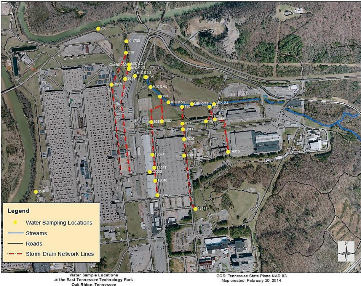
**Fig. 3.31. Storm drain (SD) networks for SDs 170, 180, 190, 200, and 210.**
