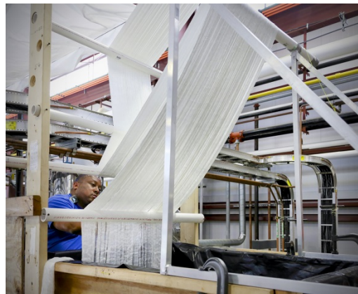
Fig. 5.3. Production of lower-cost carbon fiber at the Carbon Fiber Technology Facility.
