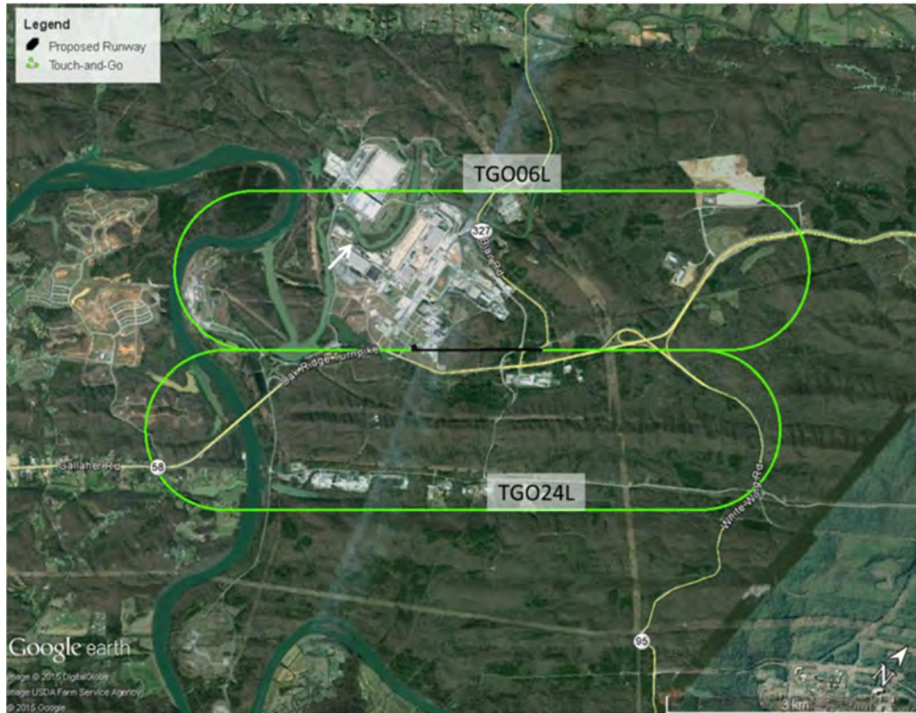
Figure 3-4. Fixed-Wing Left Turning Touch-and-go Flight Tracks
