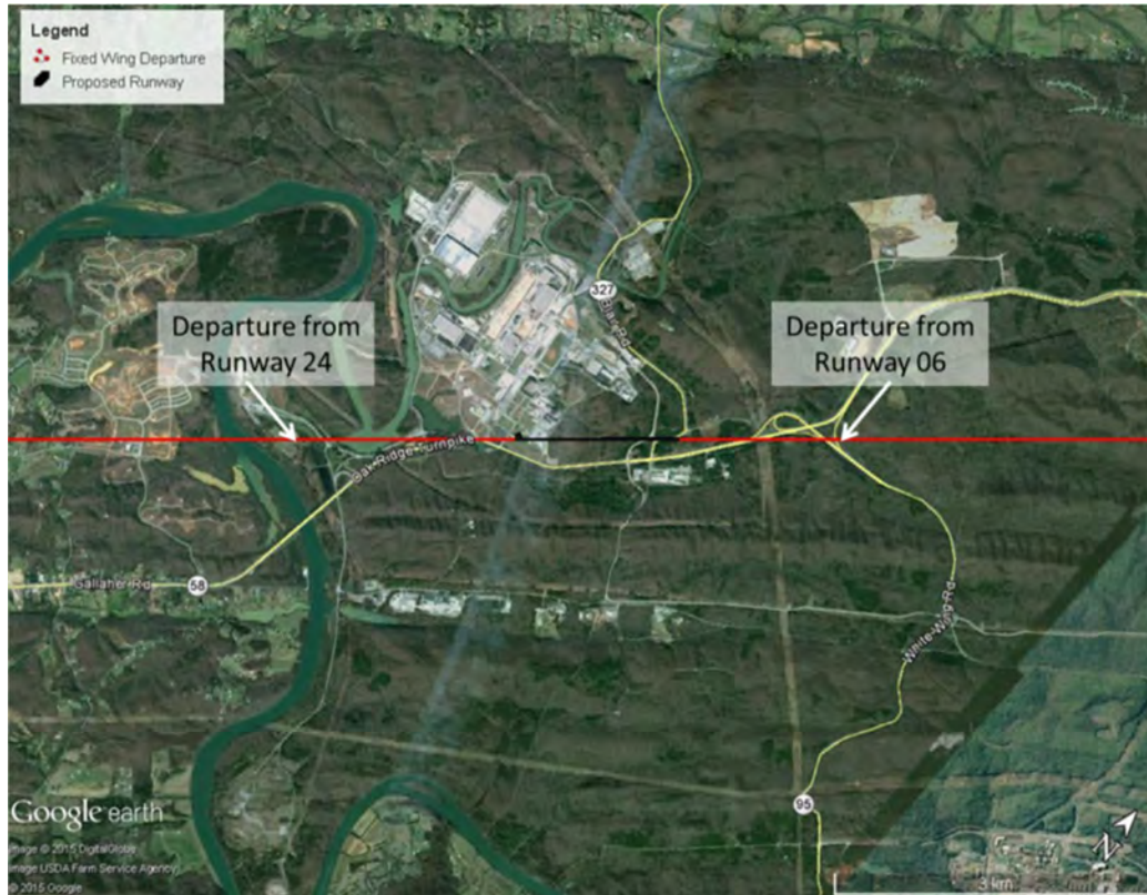
Figure 3-2. Fixed-wing Departure Flight Tracks
