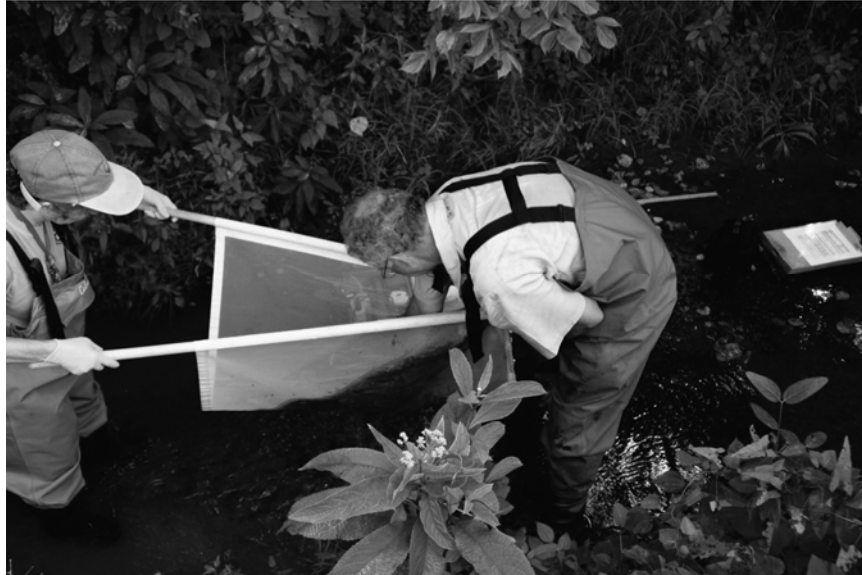
Fig. 3.54. Benthic macroinvertebrate sampling using Tennessee Department of Environment and Conservation protocols.
