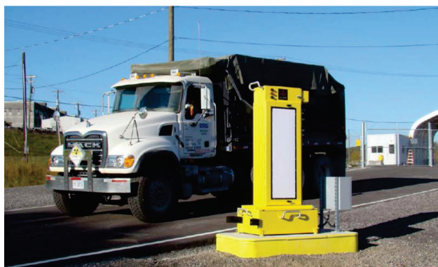
Fig. 3.6. Truck carrying a waste shipment passing through an electronic tracking station, part of the Radio Frequency Identification Transportation System, en route to the Environmental Management Waste Management Facility.
