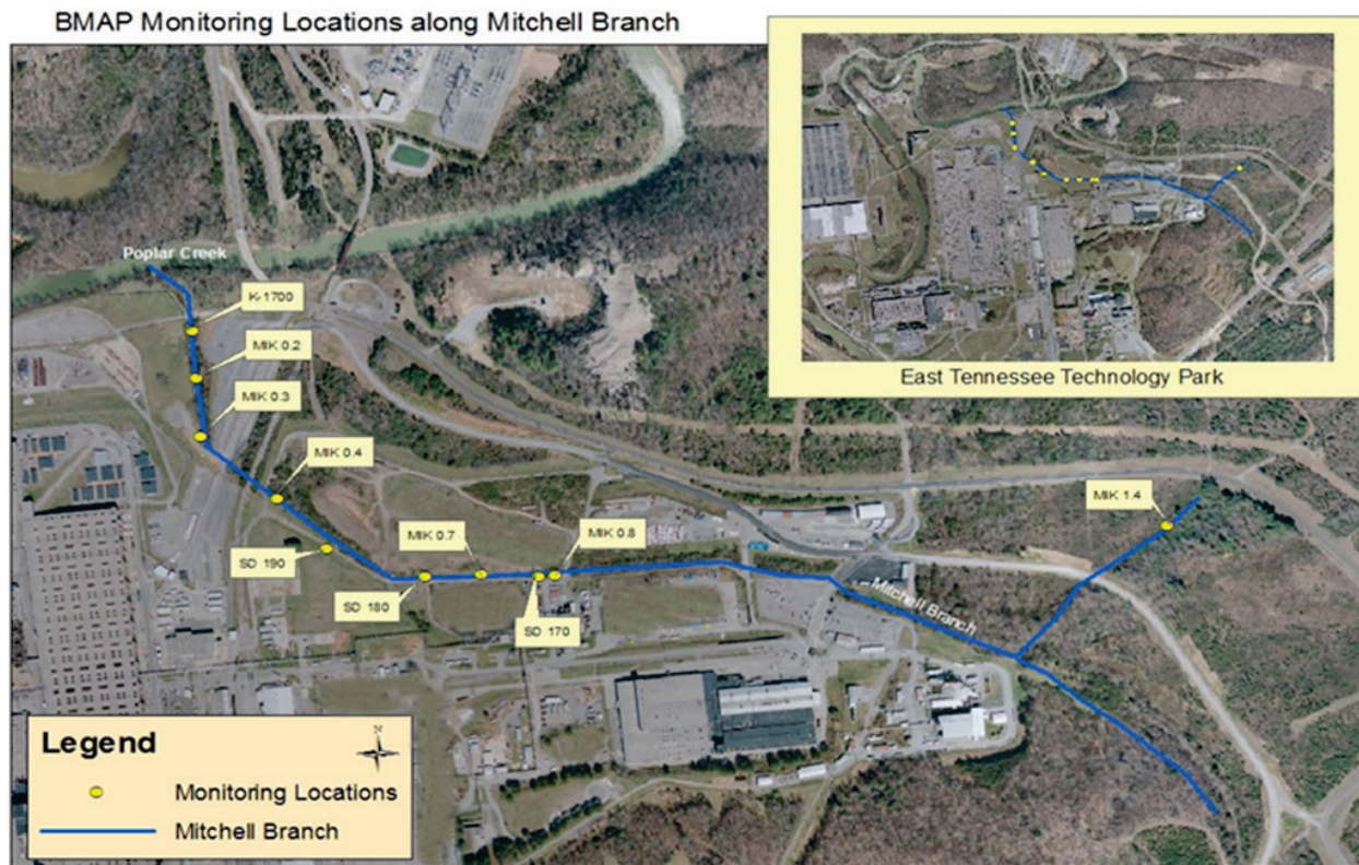
Fig. 3.44. Major storm water outfalls and biological monitoring locations on Mitchell Branch. (BMAP = Biological Monitoring and Abatement Program, MIK = Mitchell Branch kilometer, and SD = storm water outfall/storm drain.)
