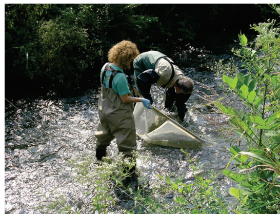
Fig. 3.52. Benthic macroinvertebrate sampling using Tennessee Department of Environment and Conservation protocols.
