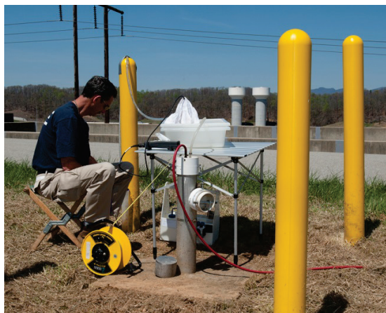
Fig. 4.37. Groundwater monitoring well sampling at the Y-12 National Security Complex. [Source: Kathryn Fahey, Y-12 photographer.]
