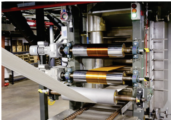
Fig. 5.2. Production of lower cost carbon fiber at the Carbon Fiber Technology Facility. [Photo by Jason Richards.]
