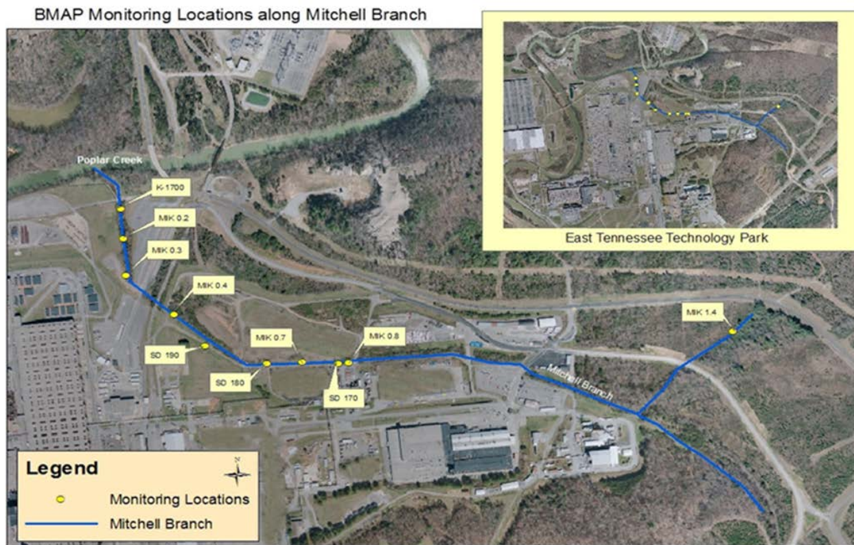
Fig. 3.40. Major storm water outfalls and biological monitoring locations on Mitchell Branch. (BMAP = Biological Monitoring and Abatement Program, MK = Mitchell Branch kilometer, and SD = storm water outfall/storm drain)
