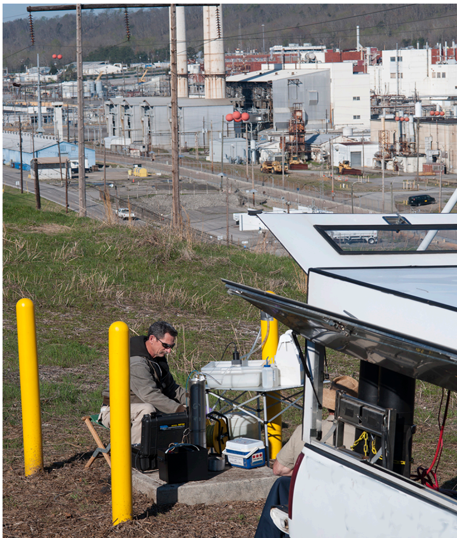
Figure 4.27. Groundwater monitoring well sampling at the Y-12 National Security Complex
