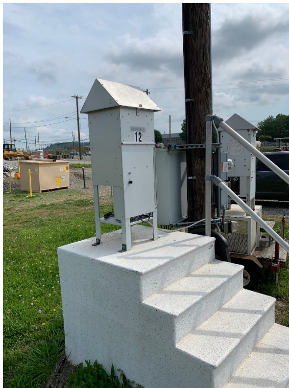
Figure 3.13. East Tennessee Technology Park ambient air monitoring station
