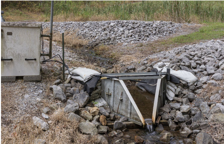
Figure 7. Leachate effluent (MCK 2.0) monitoring station downstream of passive treatment wetland.
