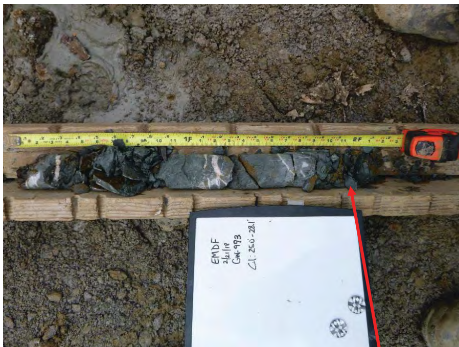
GW-993 19.8' – 35.5' Sand Pack Interval 23.0' – 33.0' Screened Interval
