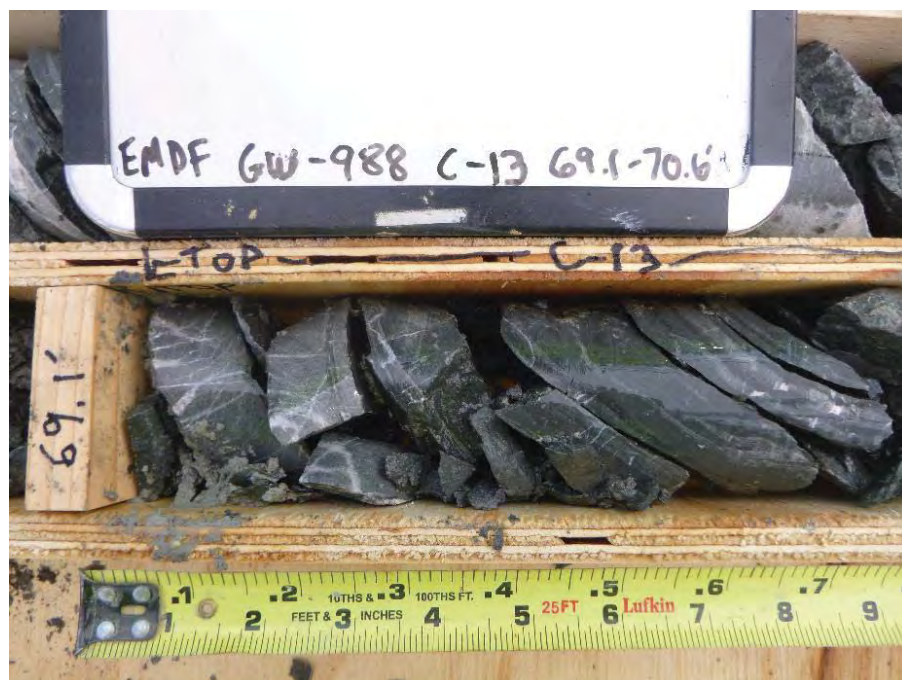
GW-988 59.6' – 74.0' Sand Pack Interval 61.9' – 71.9' Screened Interval
