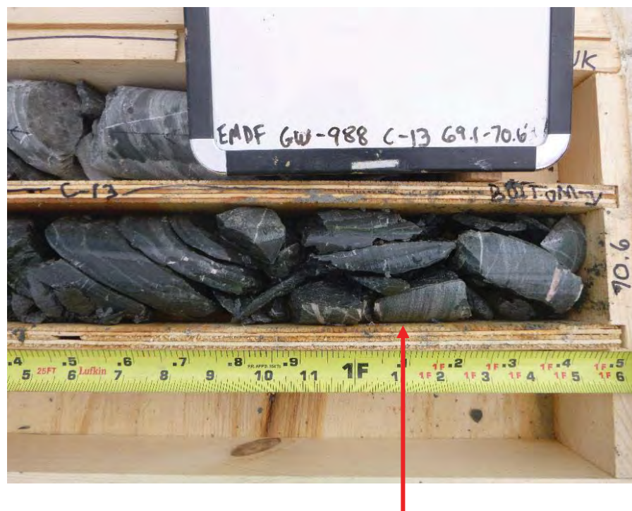
70.0' – 70.6' Vertical fracture along the bedding plane that appears to turn from 60° to near vertical. Fractures are fresh.
