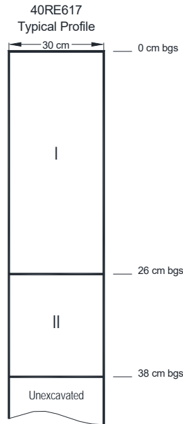
Figure 33. Typical soil profile for Site 40RE617.
